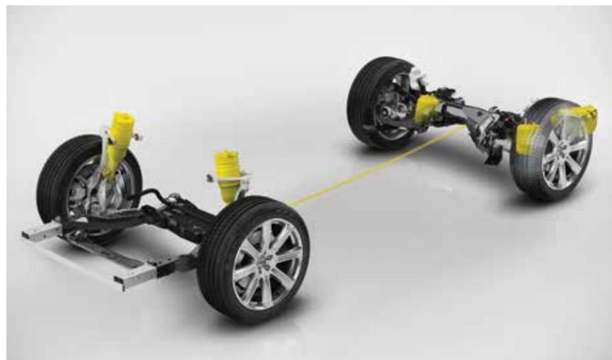
Choose the off road mode and the air suspension will raise the car by 40 millimetres. Hill Descent Control is activated at the same time: the car brakes for you on steep gradients – all you need to do is steer. The Off-road mode gets your XC90 to navigate challenging terrains – all you need to do is turn the elegant drive mode selector to the desired position.
